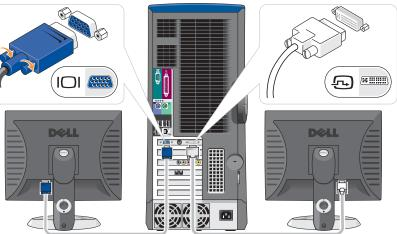
**Connect one monitor.** If your monitor has a DVI connector, plug it into the DVI connector on the computer. If your monitor has a VGA connector, plug it into the VGA connector on the computer. If your monitor has both a DVI and a VGA connector, plug only the DVI connector into the computer.
